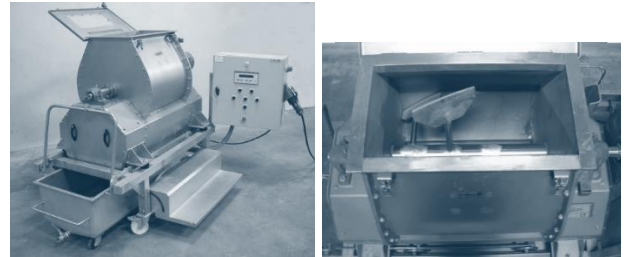
Figure 1: photographs of the mixer's exterior and interior
